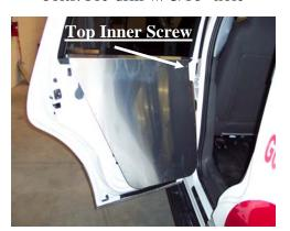
Center door panels so edges do not hang over. Attach to door with #10 x ½" stainless sheet metal screws. *Note: Window guards have holes around perimeter for permanent mounting.* <u>These holes are not used with hinge style</u> <u>window kits!</u> They also come flat in shipping.
